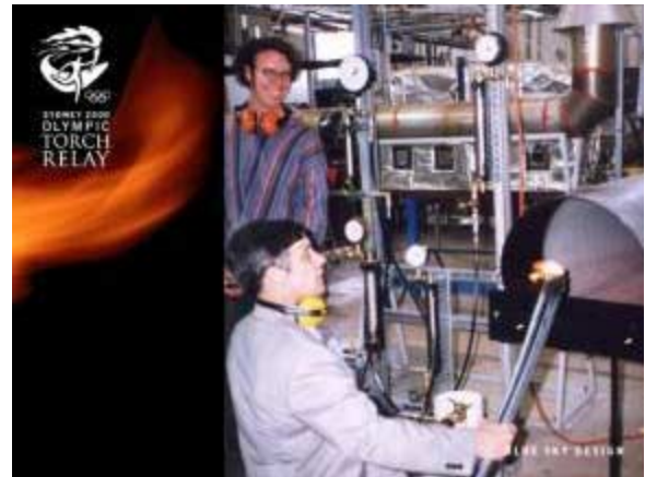
Wind tunnel testing of the torch*
