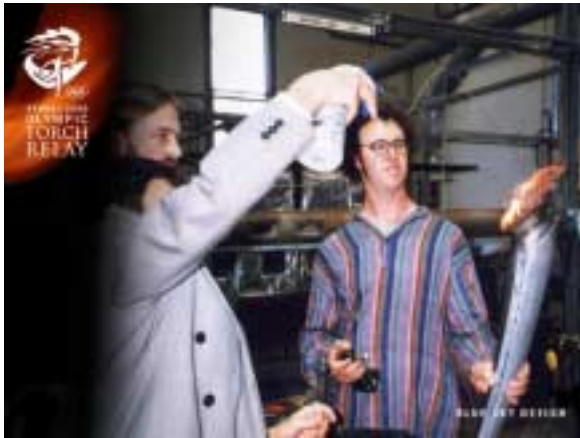
Testing of the torch for extinguishment by water*
